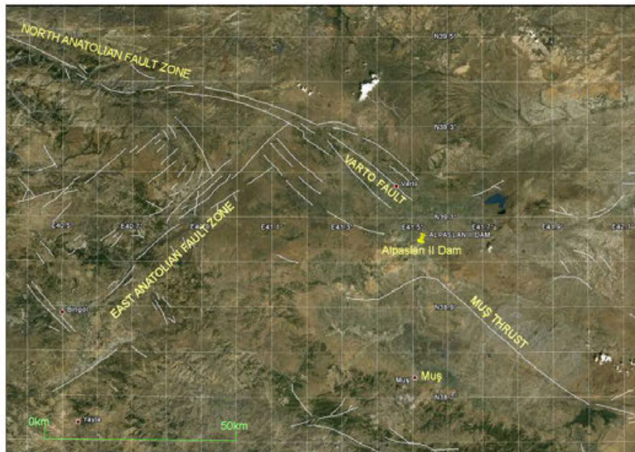
Figure 4. The main neo-tectonic features that control the earthquake hazard at the Alpaslan II Dam site.
